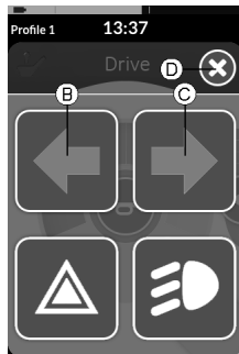
Fig. 6-31 Lighting button panel overlays screen.
