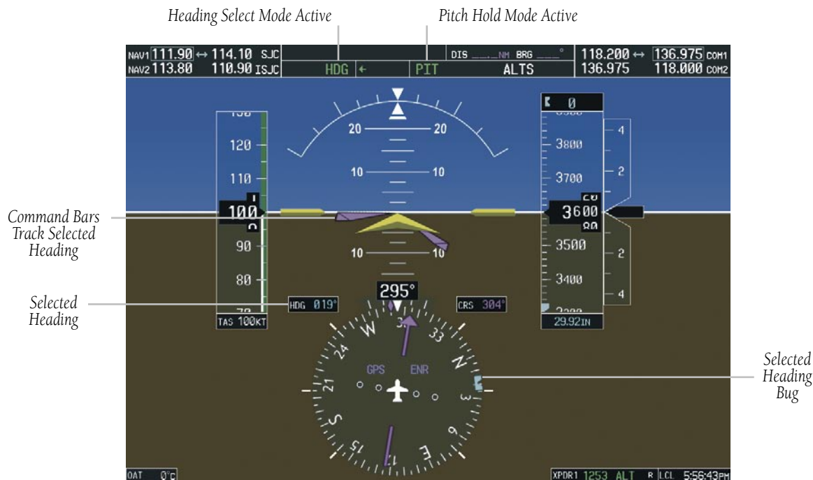
Figure 6-21 Heading Select Mode
