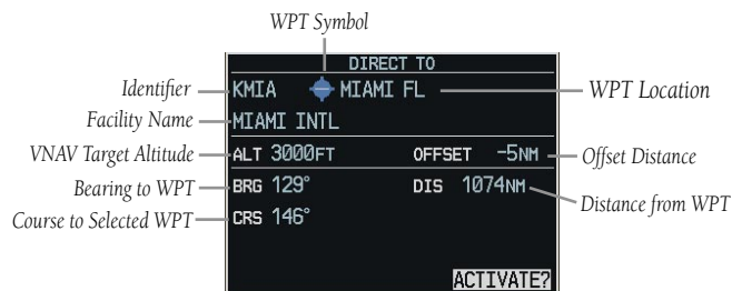
Figure 7-7 PFD Direct-to Window
