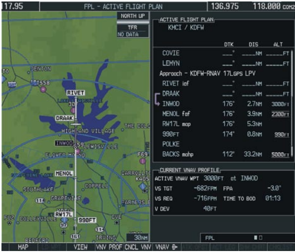
Figure 7-31 Descending Further to INWOD
