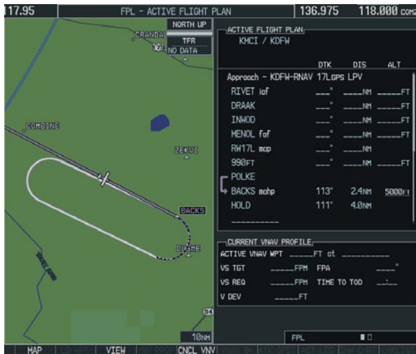
Figure 7-40 Reaching the Missed Approach Hold Point
