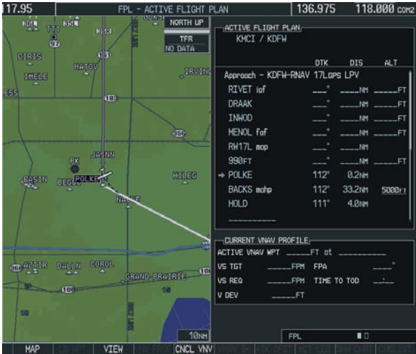
Figure 7-39 Turn Toward Missed Approach Hold Point (MAHP)
