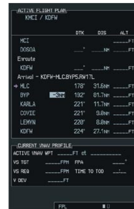
Figure 7-15 Enter Offset Distance
