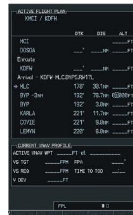
Figure 7-16 Enter Offset Altitude
