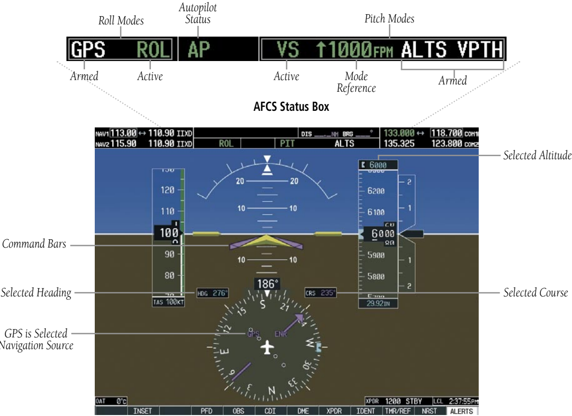
Figure 6-3 PFD AFCS Display
