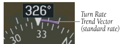
Figure 2-19 Standard-Rate Turn Indication
