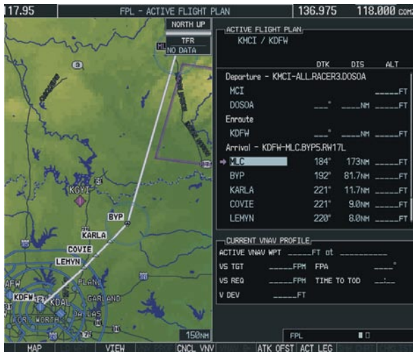
Figure 7-14 Direct-to First Arrival Waypoint
