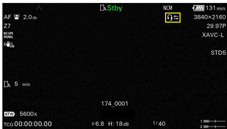
If the headset has an audio muting function, cancel muting. Adjust the intercom audio level as required, and check that communication is established.
