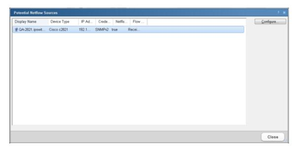
Information about devices that are potential Flow Monitor sources are displayed on this dialog along with the options for selecting a device for configuration using the Cisco NetFlow Device Configuration dialog.
