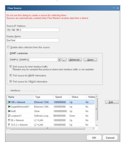
You can manually create a flow source and configure it to use SNMP to collect the following types of data:
