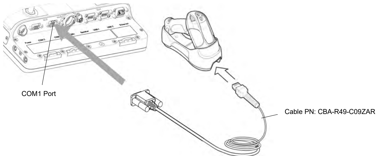
Figure 5-101 Connecting Serial Scanner Cradle to COM1 Connector
