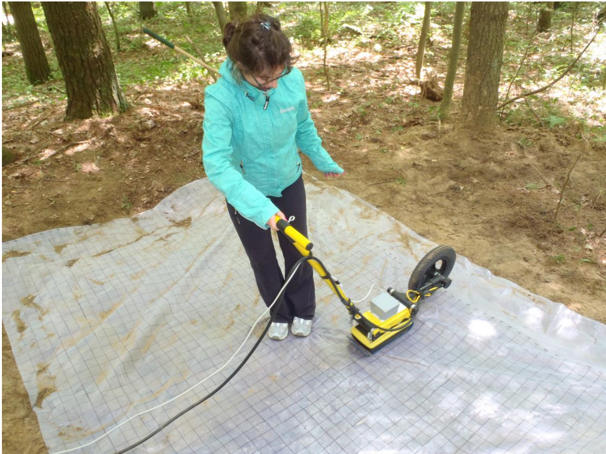
Figure Graduate student Michelle Mellon of McMaster University under the direction of Dr. Joe Boyce in the Geology/Geophysics Dept, is shown surveying a site with an accelerometer device that measures yaw, pitch and roll of the GPR antenna. The survey is being conducted to evaluate the biomass volume at the site.
