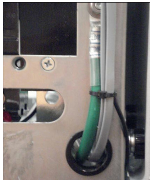
Figure 4. Route temperature sensor cables up through DCX chassis, through grommet hole and up to DCX control PCB jack locations.
