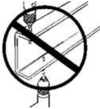
FIGURE 4-8. Frame Rail Flange Drilling Prohibited
