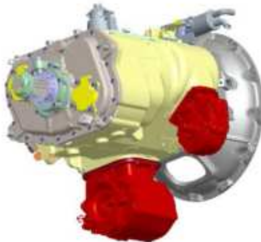
FIGURE 7-2. HD Manual Transmission
