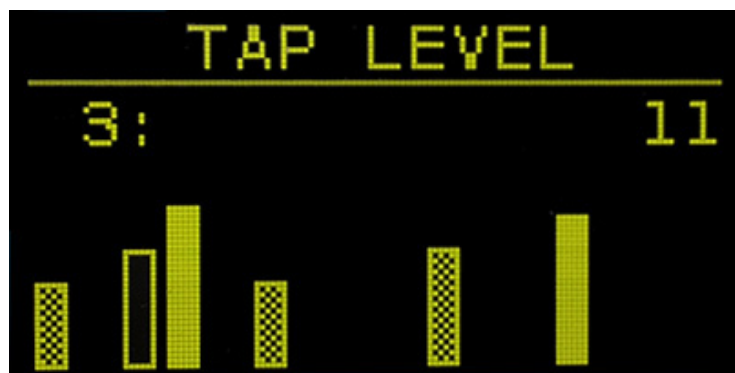
Figure 6. An example of the display when editing the LEVEL parameter for tap #3. Taps 1, 6, and 10 are muted. The tap number (3) being edited is shown in the left hand part of the second line of text, and the value of that tap's LEVEL parameter (11) is shown in the right hand part of the second line of text.
