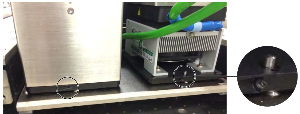
Figure 4 Each device has only 1 set screw
