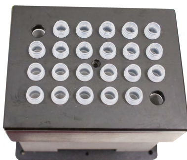
Figure 8 Hole alignment between the tube adaptor and cover
