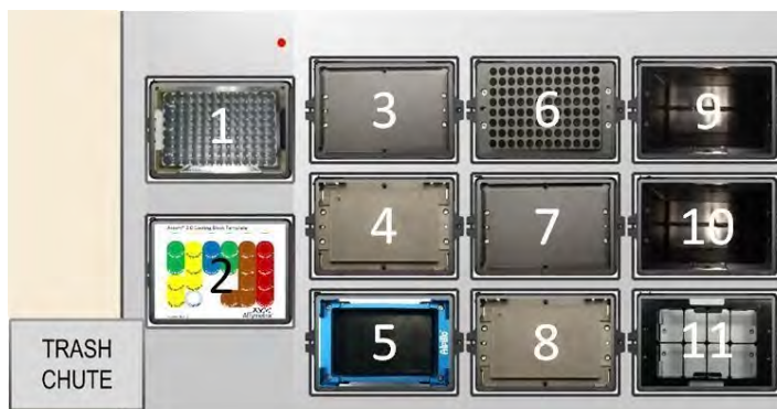
Figure 2 Axiom 2.0 NIMBUS™ Instrument Deck configuration
