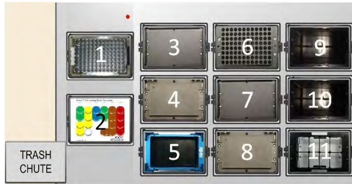
Figure 1 Axiom 2.0 NIMBUS™ Instrument Deck configuration
