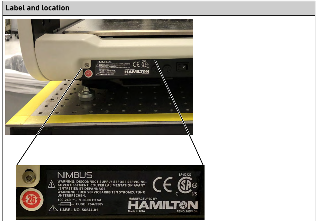
Figure 11 Warning label on the right side of the unit to the left of the power switch
