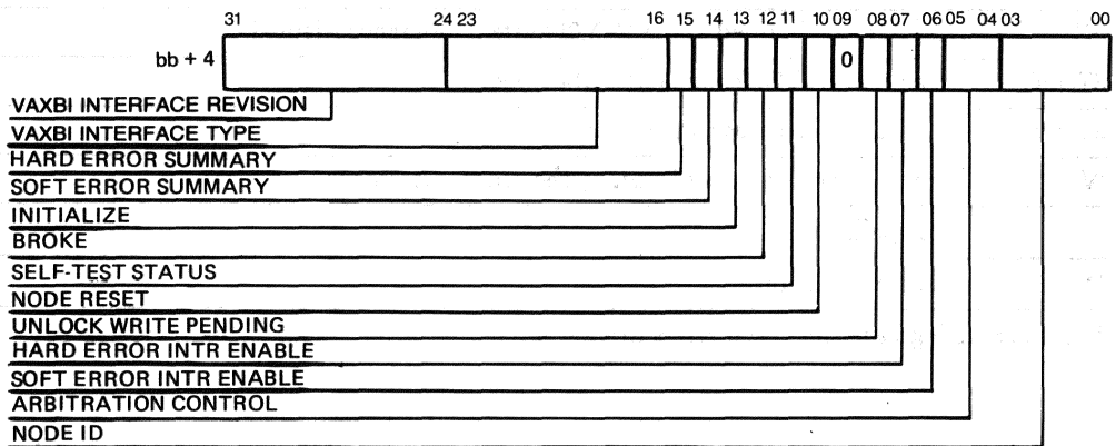
Figure 7 • VAXBI 78732 Control and Status Register Format
