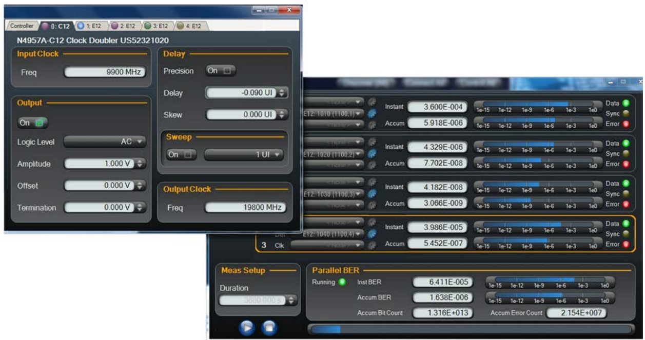
Figure 13. Decrease delay until errors occur
