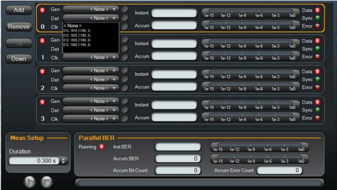
Figure 10. Adding error detectors to channels
