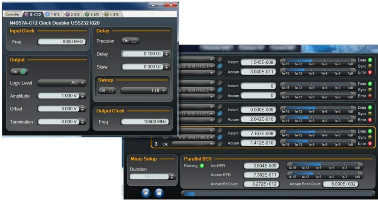
Figure 12. Increase delay until errors occur
