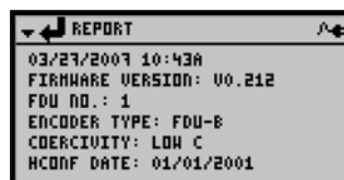
Figure 7.2b: An abbreviated version of the audit as seen on the FDU screen.
