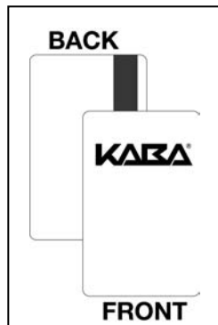
Figure 2.1: Magnetic stripe keycards (front and back)
