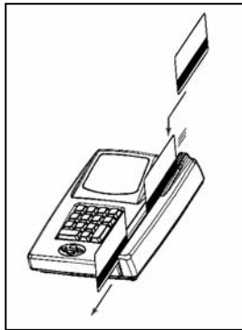
Figure 3.2.4: Magnetic stripe keycards should be placed in the slot with the magnetic stripe down and facing away from the keypad.
