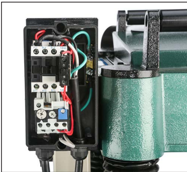
Figure 77. G0453W magnetic switch with cover removed.
