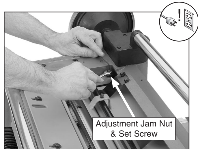
Figure 66. Example of adjusting the pressure bar height.
