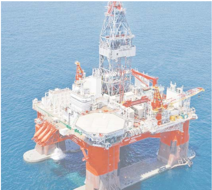
Seadrill's West Aquarius DP3 semi-sub drilling rig was built by Daewoo and utilizes a complete ABB electrical solution.
