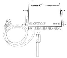
c. Connect the MULTIPAK to the Outlet: Plug the MULTIPAK input power cord into a properly grounded and compatible branch circuit outlet.
