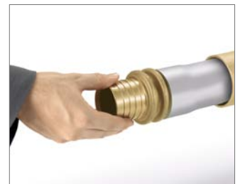
Fig. 20 4. Insert the fitting into the pipe. After a short time, the fitting should seat itself firmly inside the pipe. For RAUTHERM-FW pipe with a dimension greater than 110, REHAU lubricating agent must be uniformly applied to the pipe in the joint area.
