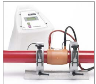
Fig. 102 Check the alignment (= insertion movement) and insertion depth.
