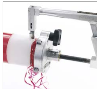
Fig. 93 Scrape the pipes twice.
