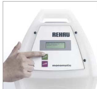
Fig. 48 10. Press the welding unit's start button and check the instructions as follows. Compare the welding parameters on the display with the values on the electrofusion fitting.
