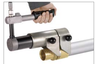
Fig. 24 8. Push the compression sleeve all the way up to the fitting collar. Once completed, pressure and temperature can be immediately applied to the joint.
