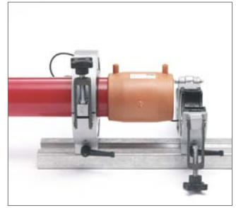
Fig. 98 Mount the universal pipe clamps as close as possible to the FUSAPEX electrofusion fitting.
