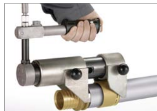
Fig. 23 7. Align the tool with the fitting and sleeve properly. Ensure the tool is sitting at a right angle to the joint. The compression jaws must be in full contact with the sleeve and fitting and be at a right angle to the connection.
