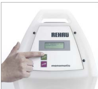
Fig. 103 Pressing the start button a second time will initiate the welding process.
