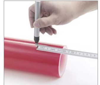
Fig. 91 Using the following table, mark the scraping area. Employ a pen in a contrasting color.
