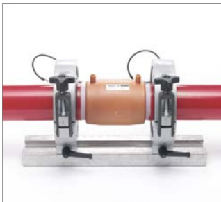
Fig. 99 Prepare the second pipe end, then slide it completely into the electrofusion fitting and secure it with pipe clamps.
