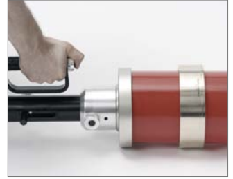
Fig. 28 3. Using the G1 expander tool expand the pipe twice rotating the pipe between both expansions by 30°. . Alternatively, the pipe can also be expanded using the expander bit (not illustrated in the Figure). Always fully insert the expander heads up to their pre-stop and align the heads properly with the pipe. Always ensure the compression sleeve is not inside the expansion area during the expansion process.
