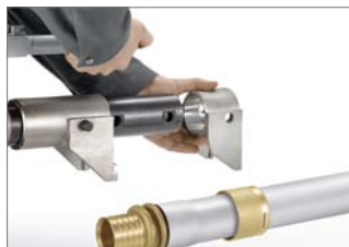
Fig. 22 6. Place the compression jaws onto the cylinder.
