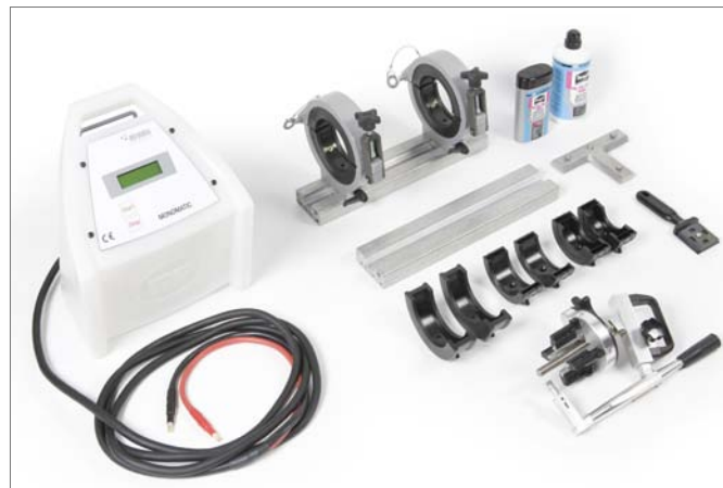
Fig. 85 Tools for creating joints
