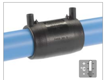
Fig. 80 The processing temperature for the pipe, fitting and welding unit must lie between -10 °C and +46 °C.
