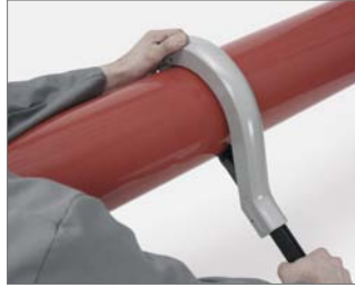
Fig. 26 Alternatively, a pipe cutter can also be used.
