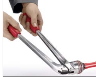
Fig. 13 3. Using the expander tool expand the pipe twice rotating the pipe between both expansions by 30°. Alternatively, the pipe can also be expanded using the expander bit (not illustrated in the Figure). Always fully insert the expander heads up to their pre-stop and align the heads properly with the pipe. Always ensure the compression sleeve is not inside the expansion area during the expansion process.
