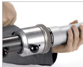
Fig. 19 3. Using the G1 expander tool expand the pipe twice rotating the pipe between both expansions by 30°. Alternatively, the pipe can also be expanded using the expander bit (not illustrated in the Figure). Always fully insert the expander heads up to their pre-stop and align the heads properly with the pipe. Always ensure the compression sleeve is not inside the expansion area during the expansion process.
