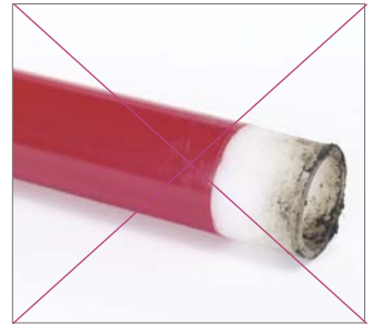
Fig. 120 The welding zone must be dry and dirt-free.
