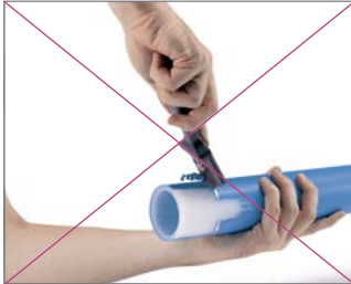
Fig. 69 Do not scrape beyond the markings.
