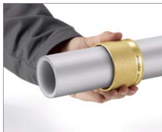
Fig. 18 2. Push the compression sleeve over the pipe. The internal chamfer must face the pipe end.
