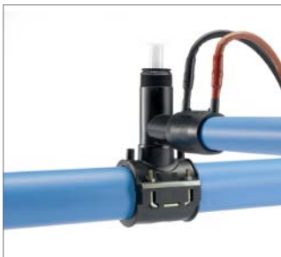
Fig. 60 8. After allowing the saddle to cool for 20 min., complete the branch pipe. Then, put the entire pipe section under pressure at the branch.
