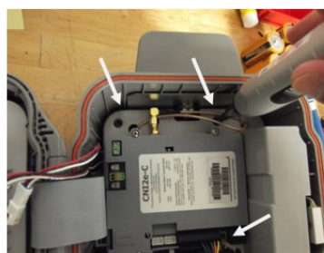
Tighten screws to 8-10 in-lbs
