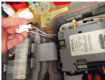
Route cables in the orientations as shown, before re-assembling HF cover
