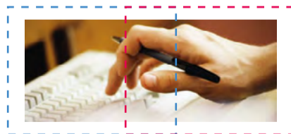
A 1200 x 480 movie to be pre-split across two overlapping 800 by 600 display areas.
