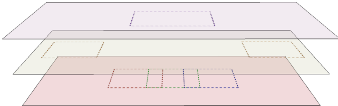
Top: The tier named "Separate", with its single high-resolution display. Middle: The tier "Sides". Bottom: The tier "Main" with the three overlapped projectors.
