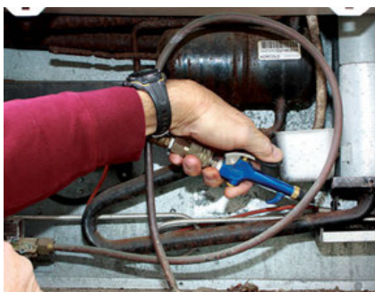
Above and below: This Norcold refrigerator's maintenance had been ignored for many years. Rust needed to be blown out of the burner assembly and flue.
