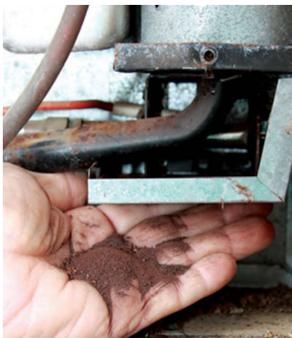
Above and below: This Norcold refrigerator's maintenance had been ignored for many years. Rust needed to be blown out of the burner assembly and flue.
