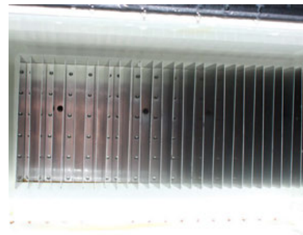
Be sure the refrigerator's interior cooling fins are intact and evenly spaced for maximum cooling output.
