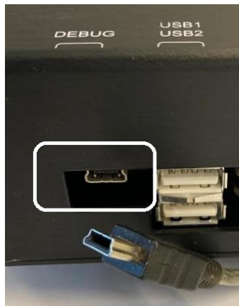
Figure 11: PPC Serial Connection
