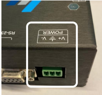
Figure 7: PPC Power Supply Connector
