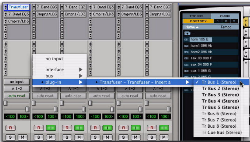
Figure 6. Selecting Transfuser Bus 1 as the input for an audio track in Pro Tools
