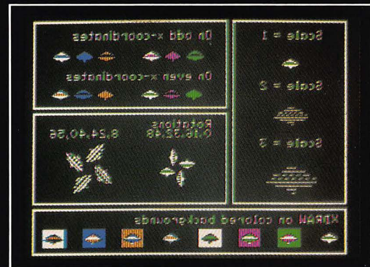
Applesoft shapes. Shapes can be scaled, rotated, drawn and X-drawn.
