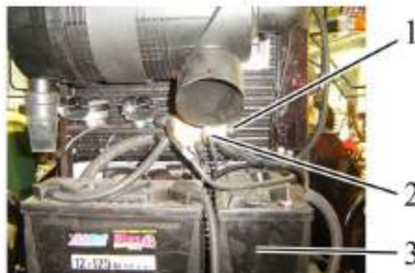
Figure 2.2.5 – Assembly the accumulator battery manual disconnect switch
