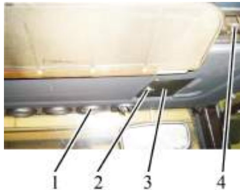
Figure 2.17.1 – Access to cutout fuses located in the upper compartment of the cab
