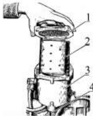
1 – filter cap; 2 – filter cartridge; 3 – filter housing; 4 – plug.
