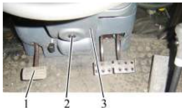
Figure 2.17.3 – Access to cutout fuses located under the dashboard
