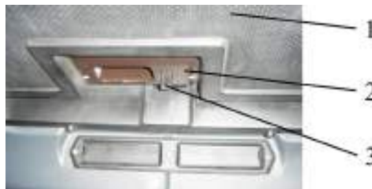
1 – hatch; 2 – board; 3 – detent.
