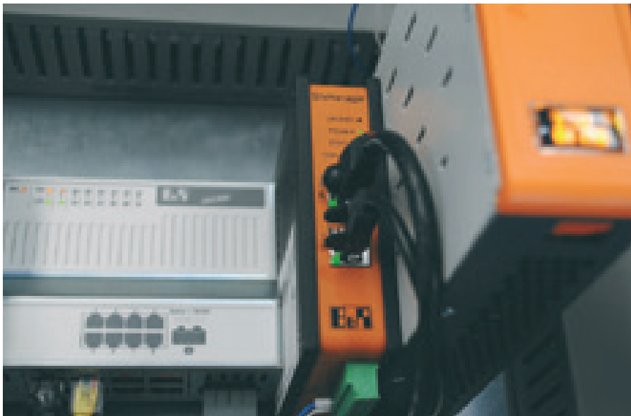
SiteManager is a small, secure, Internet-enabled modem that connects the machine in the field, via the installed PLC, to the Internet and the GateManager server.
