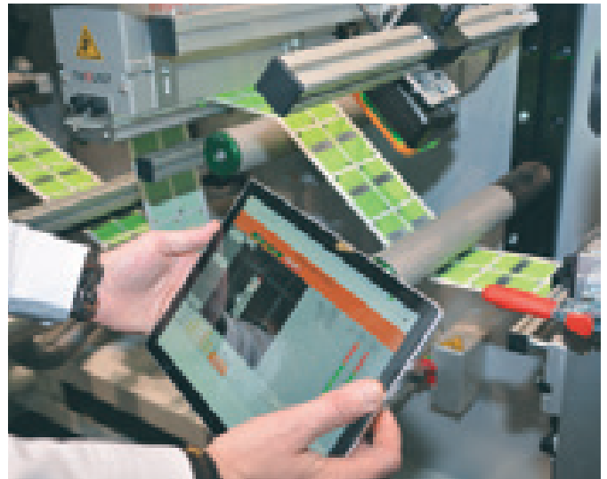
With HTML 5 and mapp Technology, Spilker is able to offer users both traditional HMI operation and web-based operation using smartphones or tablets.
