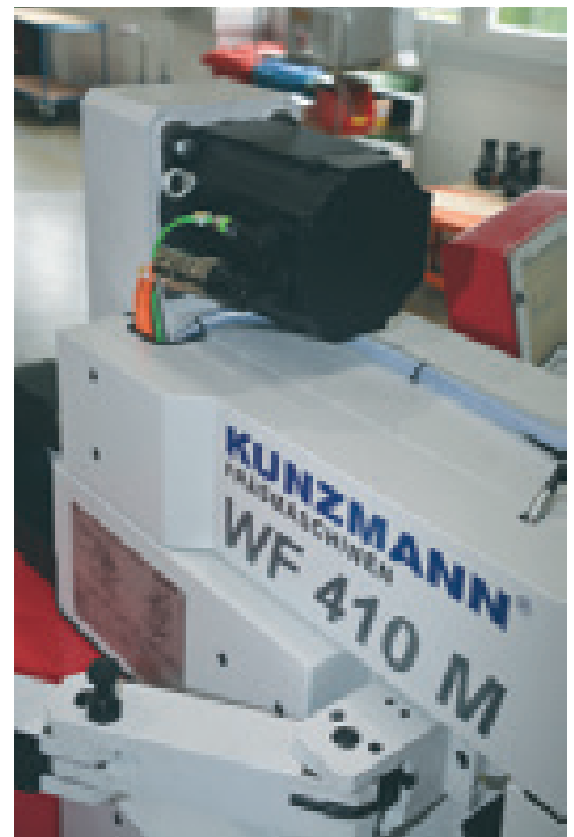
Powerhouse: By replacing an induction motor with a fanless B&R servo motor, Kunzmann cut the space required for the spindle motor nearly in half.
