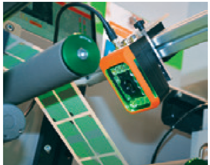
The B&R Smart Sensor used by Spilker provides position values for each label in real time, which are then used to control the system's die cutters.
