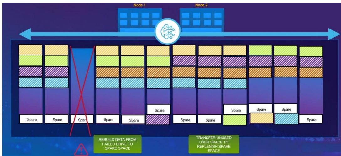
Figure 26 Rebuild data chunks to spare space after drive failure and replenish spare space with unused user space
