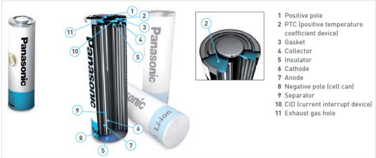
Figure 3-1. Images of a Panasonic 18650 cylindrical Li-ion battery cell.
