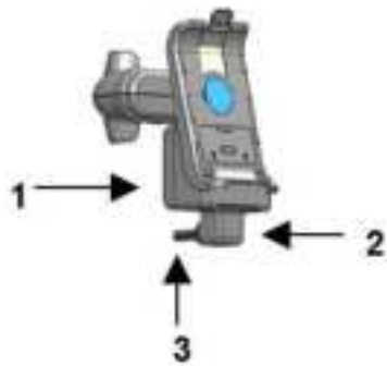
Figure 2.4. Mini-Cradle with Integrated Power Supply
