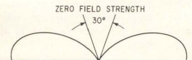
FIG. 3—Absence of display over region of zero field strength enables aircraft to pinpoint beacon
