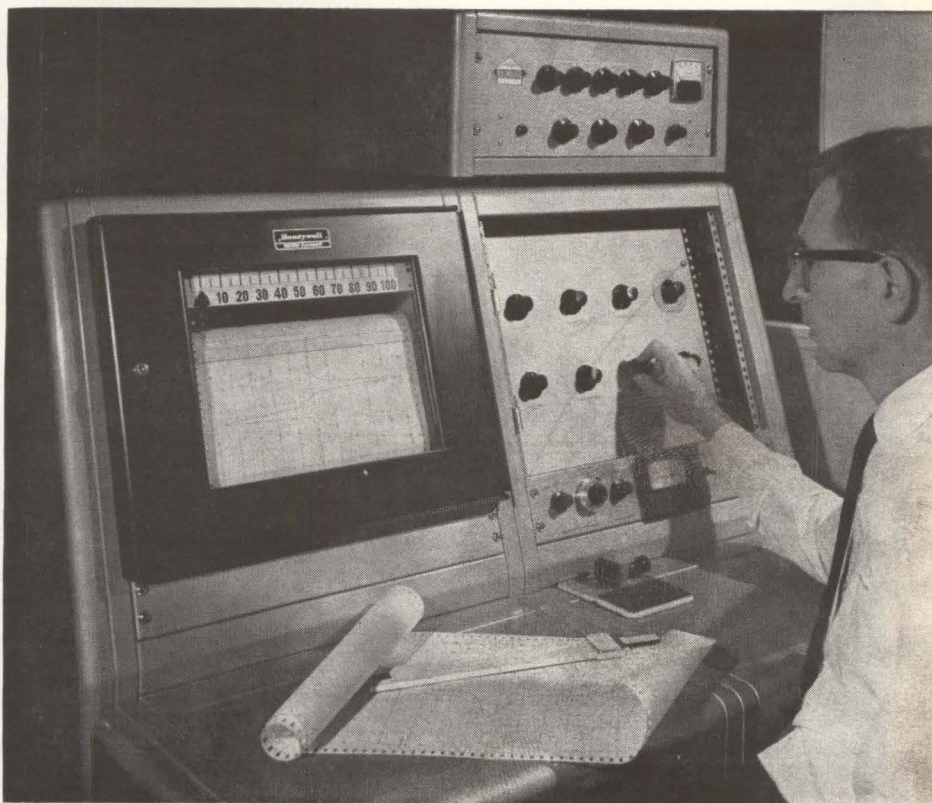
Research chemist investigates moisture content of living tissue using Schlumberger's model 106 nuclear magnetic resonance analyzer
