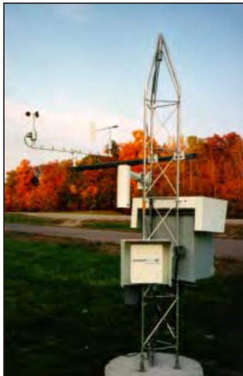
Weather Station with 10' Tower
