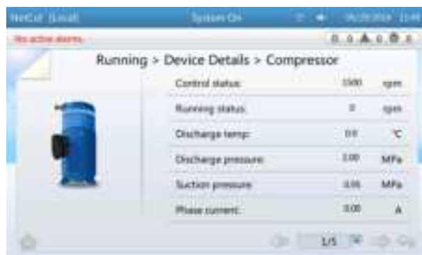
Figure 4-34 Compressor running status
