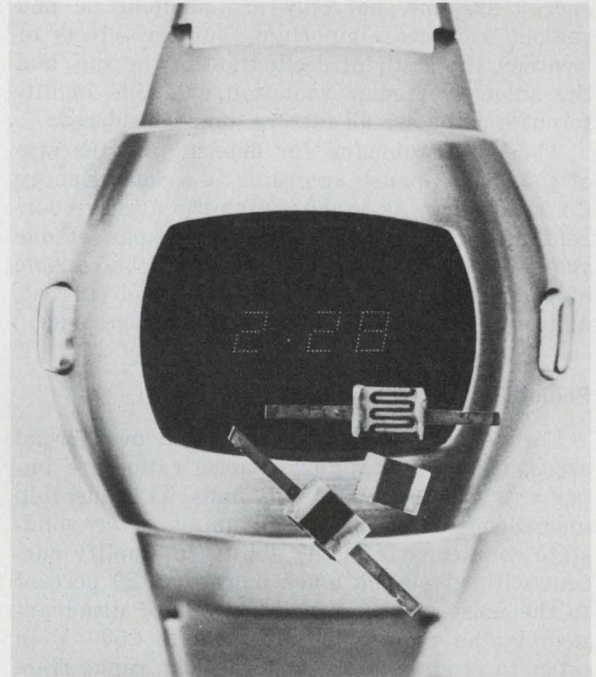
Watching brightness levels is the job of NSL's 200 series CdS/Se photocells. The combination of materials offers the speed and sensitivity of CdSe and the stability of CdS. These photoconductive cells operate over a spectral range of 630 to 690 nm—also well suited for detecting light from GaP and GaAsP emitters.
