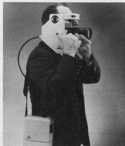
Use of standard ICs helped reduce the Microcam color TV camera to half the size and weight of competing units.
