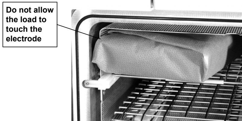
Figure 17. The Load Should NOT Touch the Electrode.
