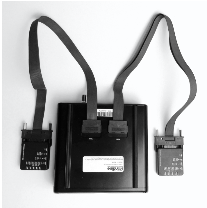
Figure 2.10 - HCI Pods Installed on Sodera
