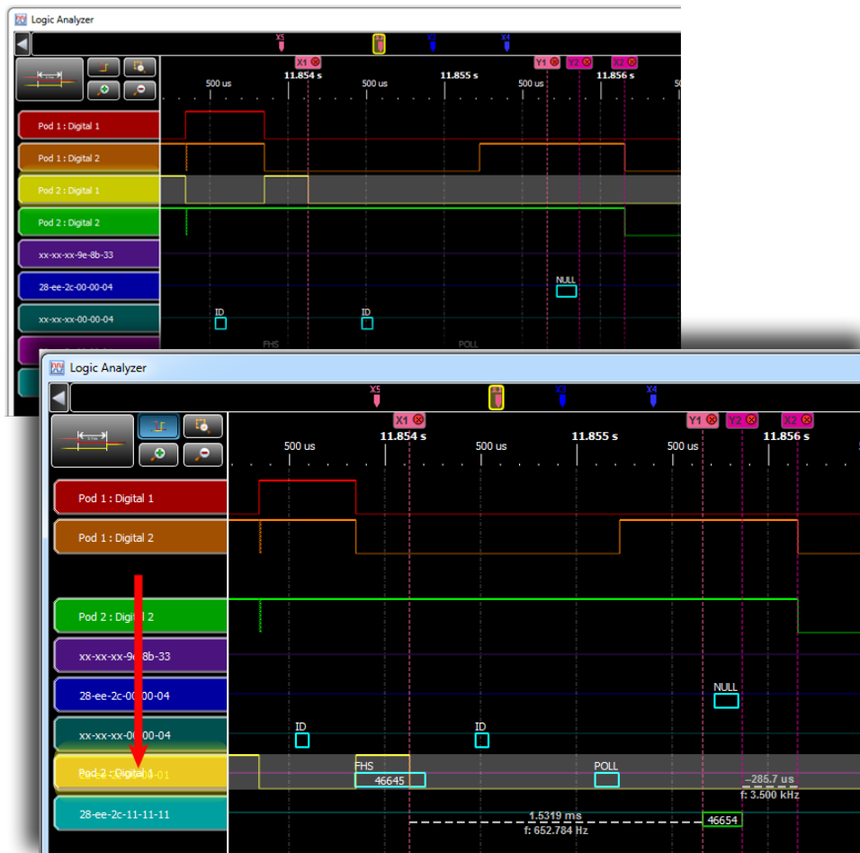
Figure 4.124 - Logic Analyzer Overlay Signal Example
