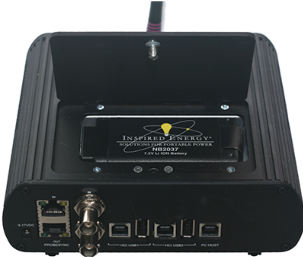
Figure 2.4 - Sodera Battery Compartment with Cover Opened
