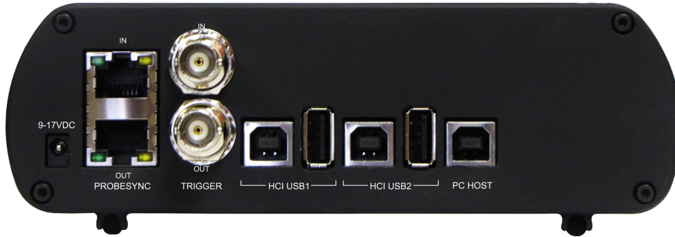
Figure 2.2 - Sodera Rear Panel Connectors
