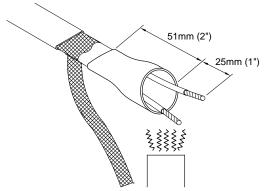
2 Slide one 13mm (0.5") diameter, 51mm (2") length shrink tube over both pigtail leads leaving approximately 25mm (1") of each pigtail lead exposed. Shrink with heat gun until completely shrunk.
