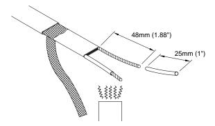
O Slide one 3mm (0.125") diameter, 25mm (1") length shrink tube over each bus wire leaving approximately 13mm (0.5") of each bus wire exposed. Shrink with heat gun until completely shrunk.
