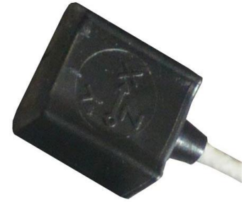
Tri-axial accelerometer uses 3 channel inputs
