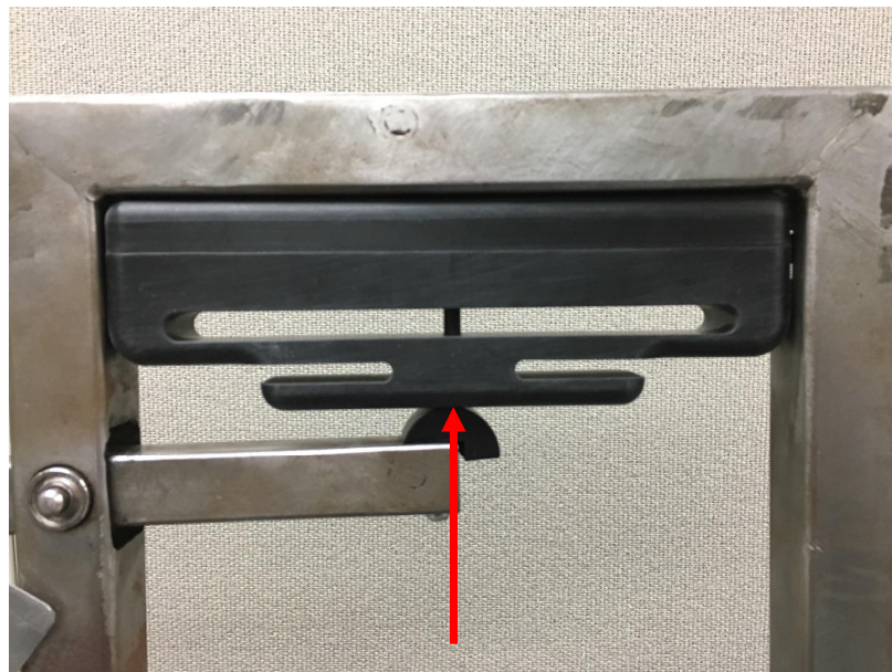
Figure 2: Delrin handle within the test fixture. Red arrow indicates placement of applied force which is at a single point; not distributed across the handle.
