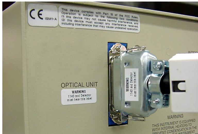
Figure 2-2 Attaching an Optical Unit to the UA-6
