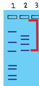
Figure 5: Measure distance migrated from the lower edge of the well to the lower edge of each band.
