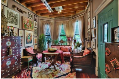
Figure 7 Example of excessive fire load
