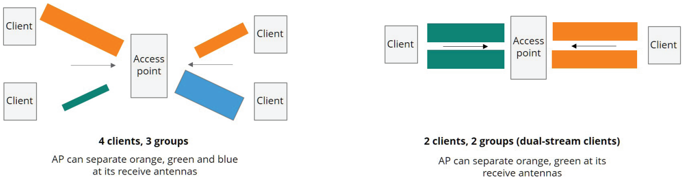
Figure 39: Uplink multi-user MIMO transmission
