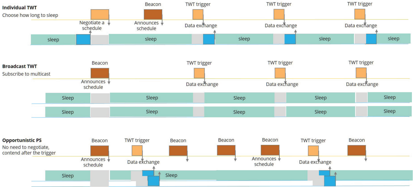
Figure 29: TWT power-save options in 802.11ax
