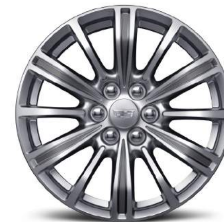
18-IN. ALUMINUM WITH BRIGHT MACHINED FINISH AND LIGHT ARGENT ACCENTS Standard on XT5 Luxury
