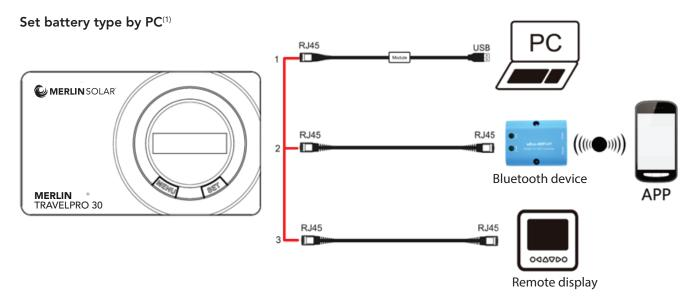
(1) Only Sealed, Gel and Flooded via the LCD. The battery type of User can be set via the PC software, APP software and MT50.
