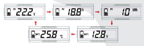
Display: PV voltage, PV current, PV power, Battery voltage and Battery temperature
