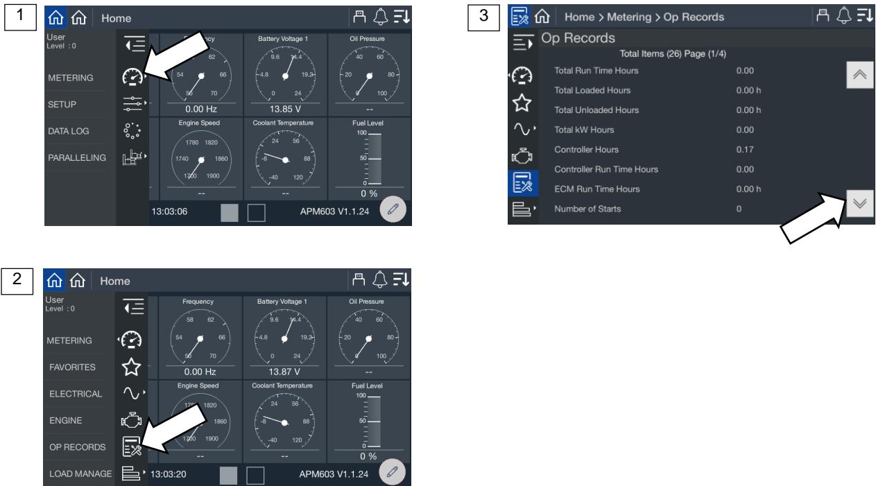
Figure 42 Metering Screen, Operation (Op) Records
