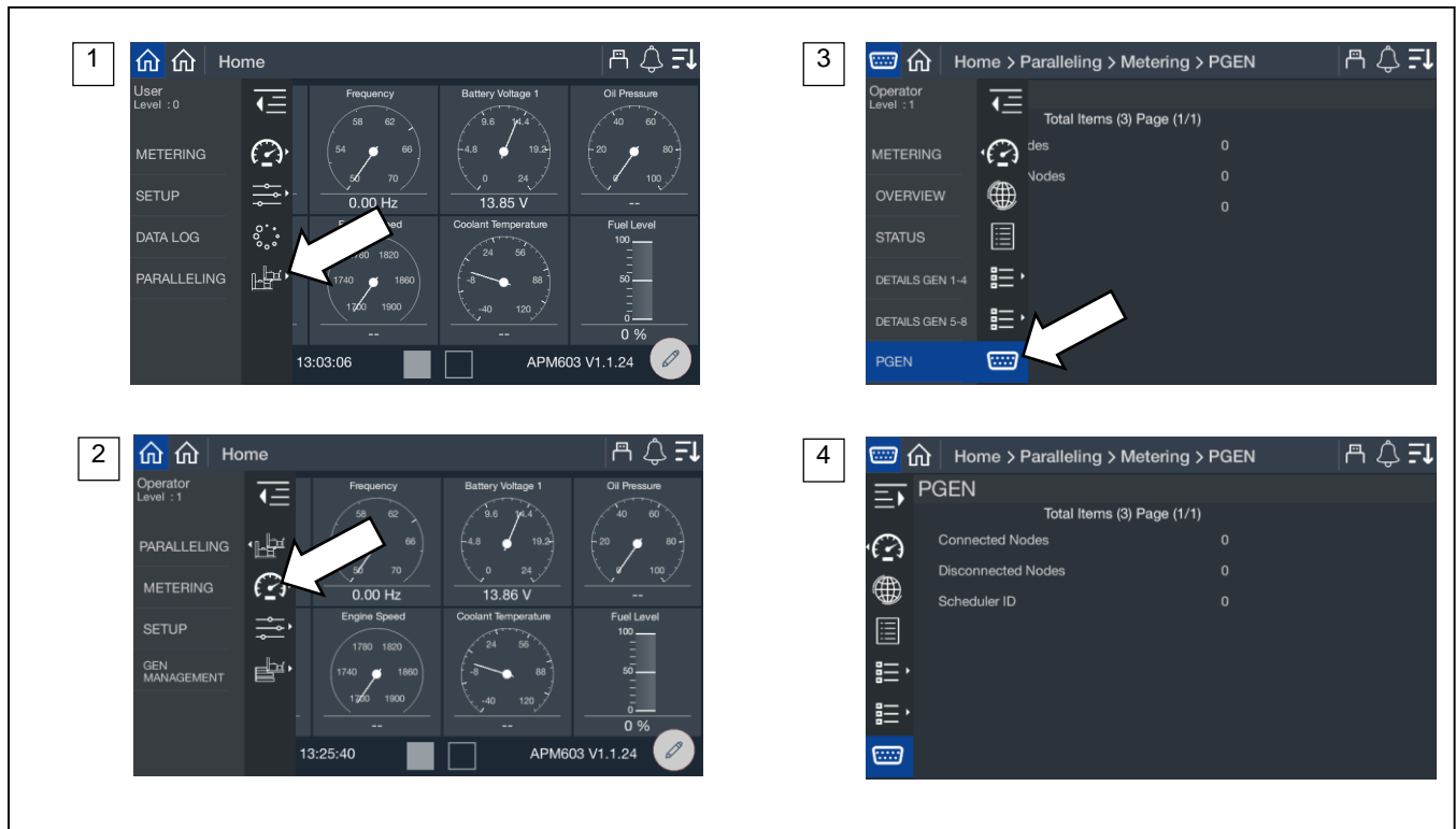
Figure 69 Paralleling, Metering, PGEN
