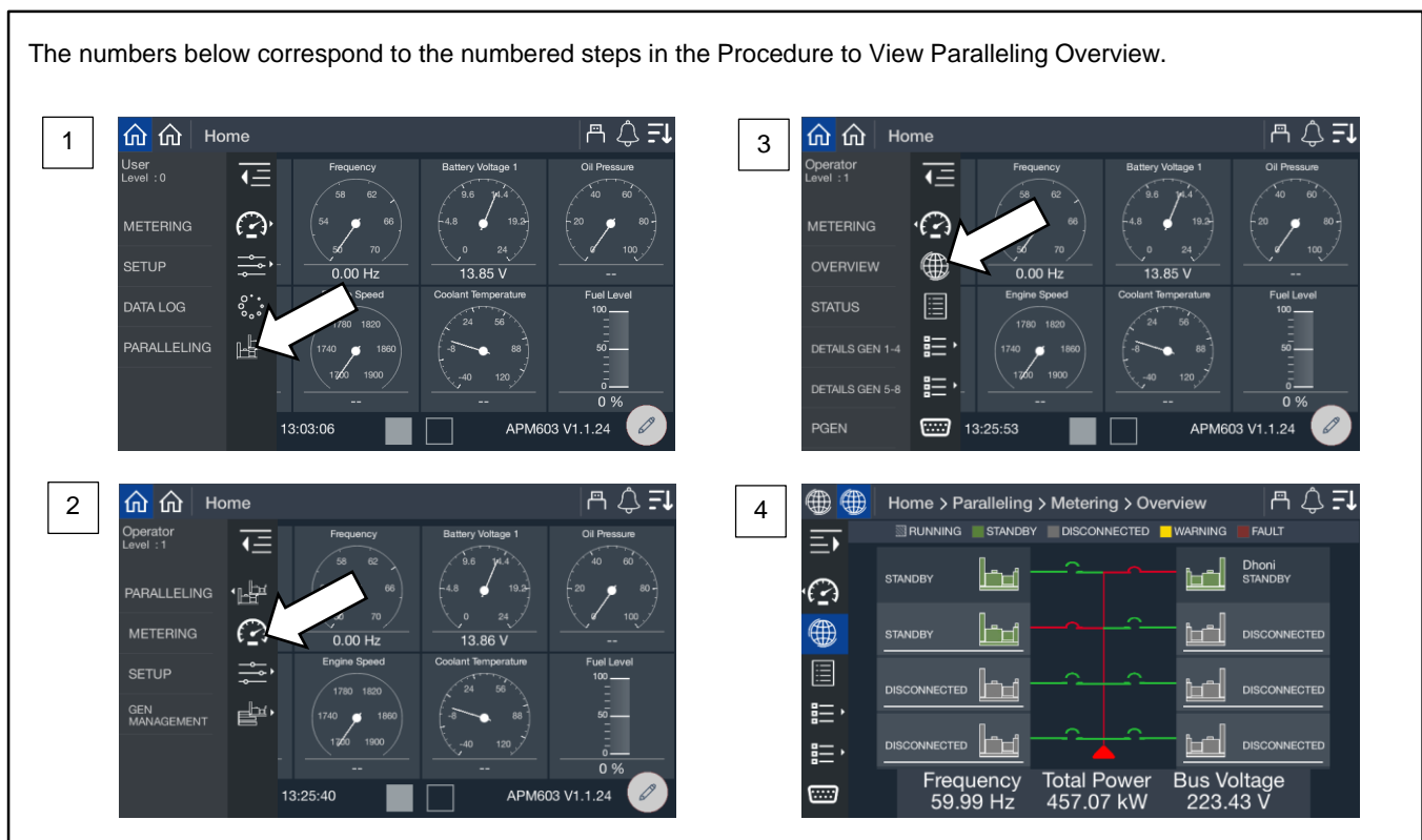
Figure 64 Paralleling, Metering, Overview Screen
