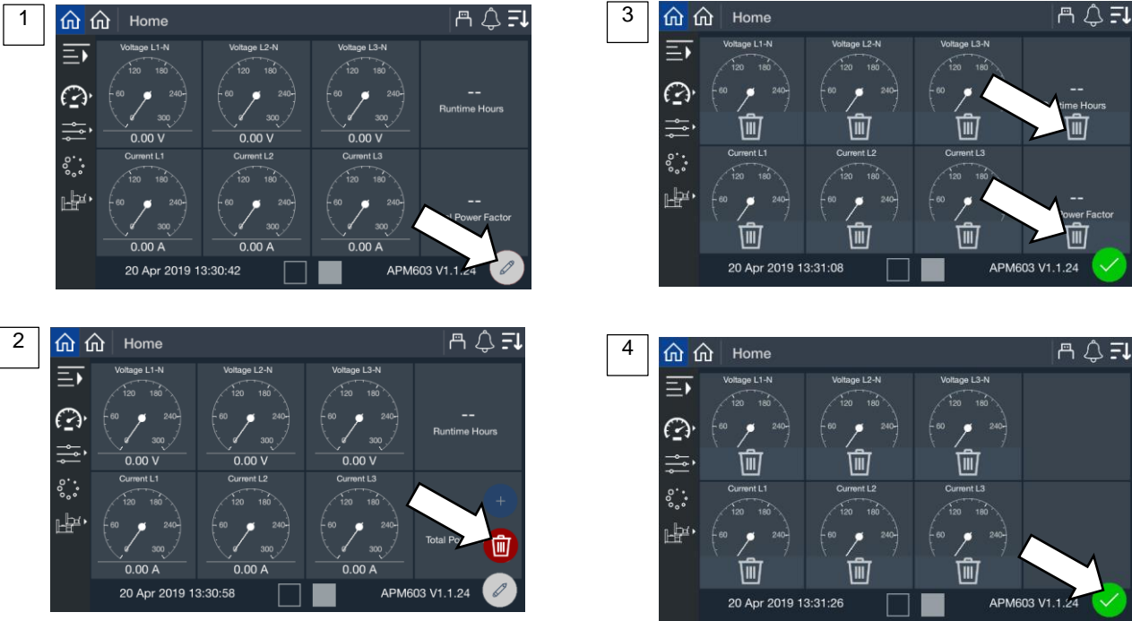
Figure 20 Removing Gauges from the Home Screen
