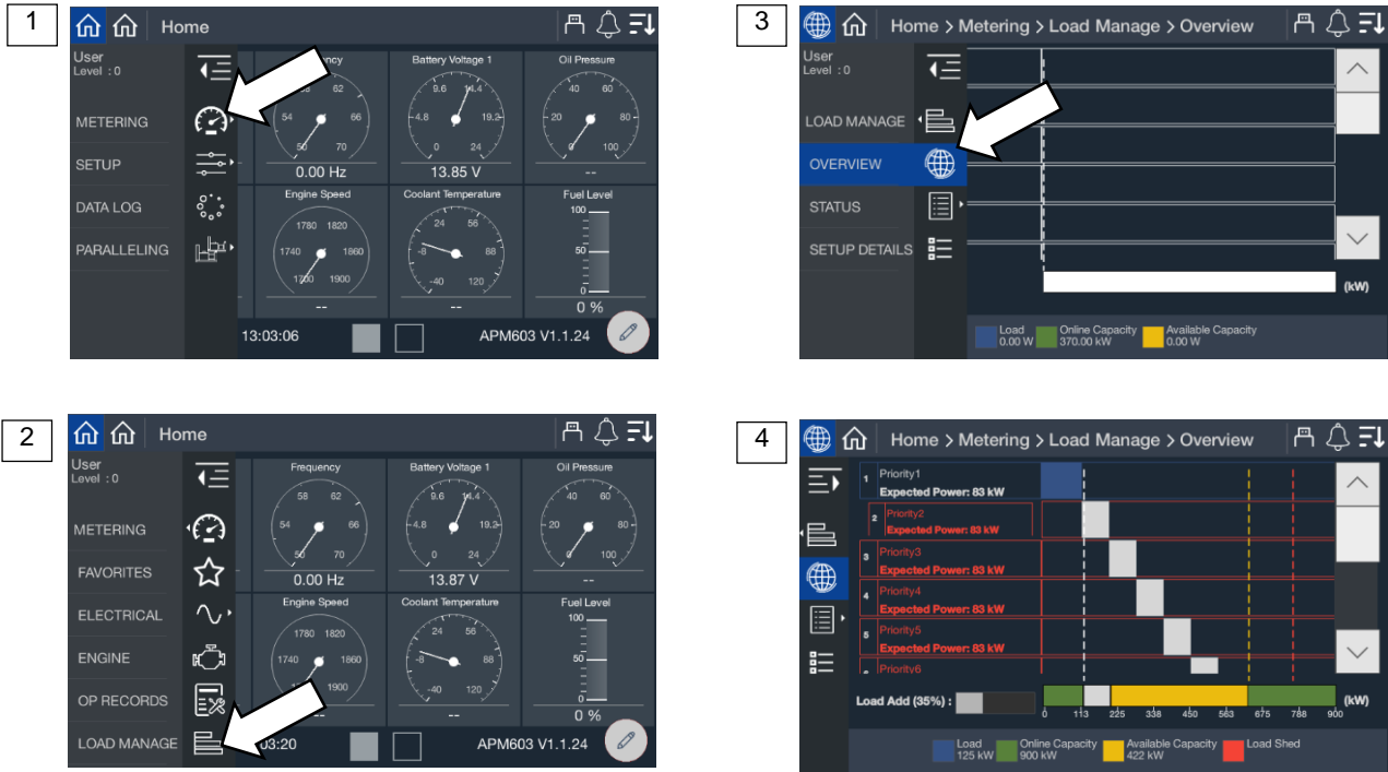
Figure 44 Metering Screens, Load Management Overview
