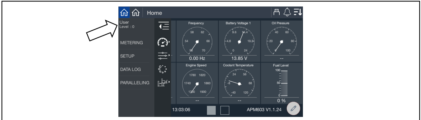
Figure 6 Access Level Indication
