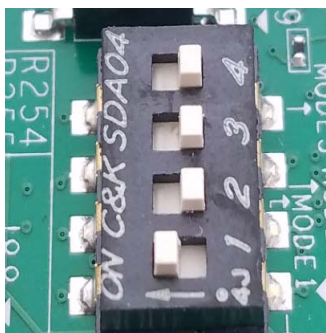
Figure 5-7: SW6 Switch Settings for SD Boot Mode
