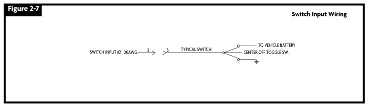
Unused switch input pins should be fitted with Deutsch pin sealing plugs. These are included in the connector kit from Akron Brass.
