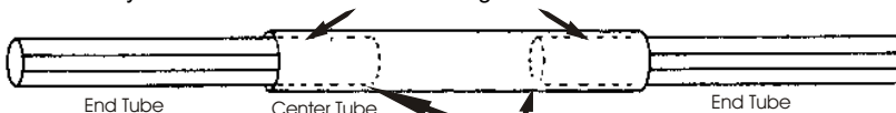
Fig. 3 Insert both end tubes equal distance into center tube and mark on center tube where inner tubes end
