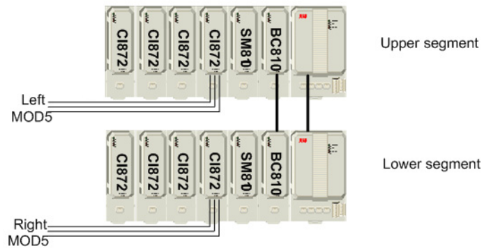
Figure 35. Maximum Configuration Using HI Controller
