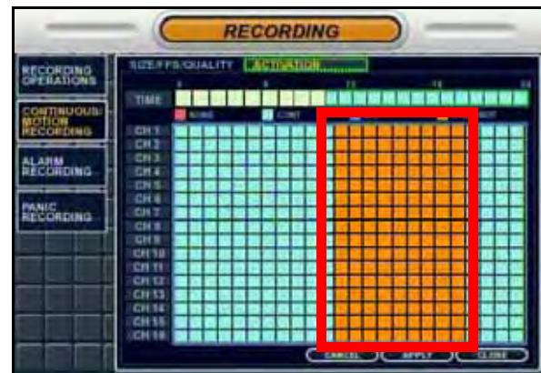
Figure 28.6 Multiple blocks set for Continuous+Motion
