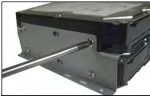
Figure 41.5 Insert the new HDD and secure with screws
