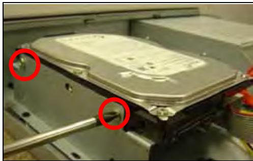
Figure 41.4 Unscrew the four chrome screws on the hard drive bracket.
