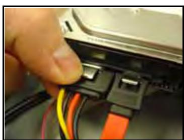
Figure 41.2 Unplug the SATA data and power cable from the hard drive.
