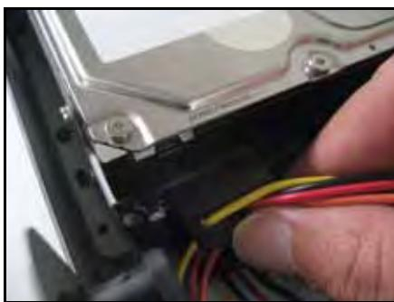
Figure 41.6 Connect the SATA power and data cables
