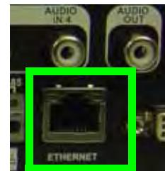
Figure 1.2 Connect an RJ45 network cable into the ETHERNET port.
