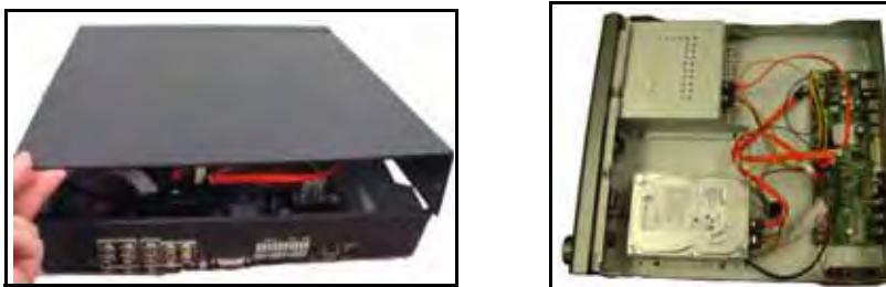
Figure 41.1 Gently remove cover. Be careful of sharp edges on the cover.
