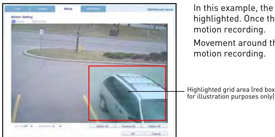
Figure 35.6 Adjusting motion sensitivity.
