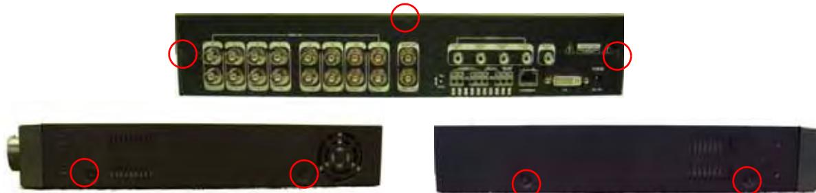
Remove the screws on the side panels and the rear panel. Gently slide cover off.
