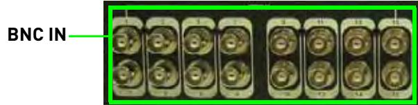
Figure 1.0 Connect BNC cameras to the system (\*16-channel shown).
