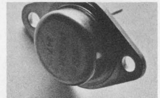
The first 3-amp positive IC regulator.
