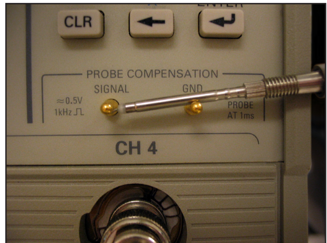
Figure 4. Calibrating a scope probe.
